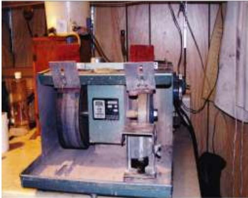
**Raytec Lab Cabber** with sanding drum, 100 grit diamond wheel, Diamond disk, grinding table, saw table, 3 splash shields, variable speed (pulley crank) and water tank (drip cool)
